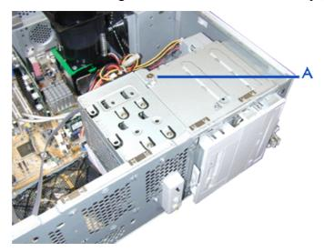
Figure 4 - 16 : HDD Bracket Screw
